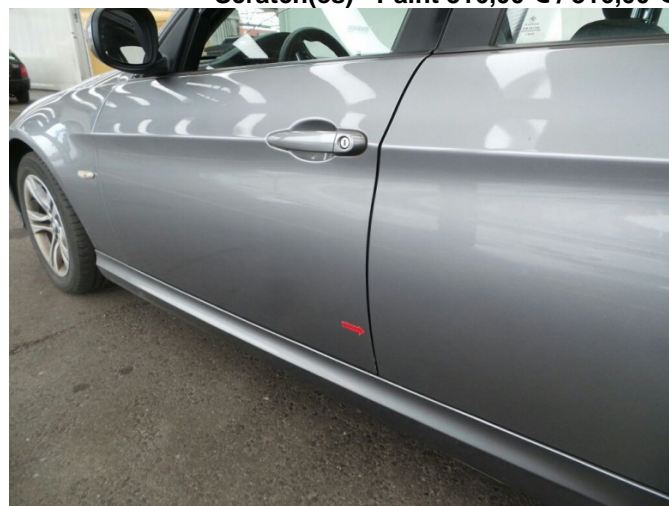
3. Front door - left Wear and tear - Without repair 0,00 € / 0,00 €
