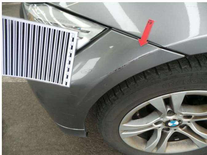
1. Front bumper Scratch(es) - Refurbish and paint 0,00 € / 0,00 €
